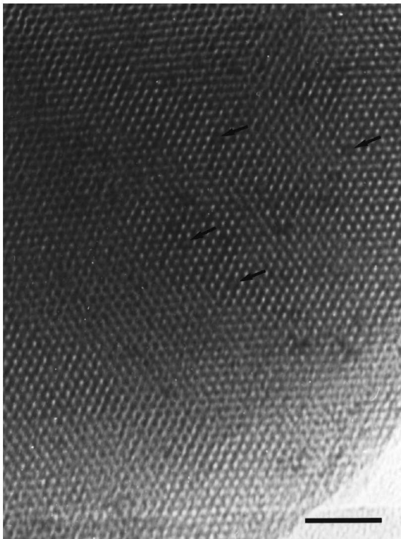
Fig. 5. TEM image of Fe/M41-12 observed on Hitachi H-1250M with acceleration voltage of 1000 kV. The arrows indicate presence of iron oxide particles in the pores of the support and the bar in the figure shows 30 nm.
